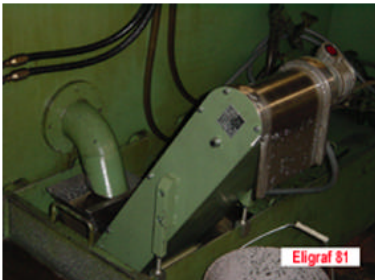
1) Magnetic conveyor mod. L100 with plan in stainless steel
